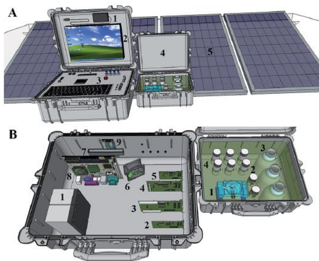
Fig. 3 The PG004 (A), 1: GPS, 2: touchscreen, 3: panel with an optional keyboard, keys, and command bottoms, 4: flow module, and 5: solar boards. The internal view of the PG004 (B), 1: 12 V batteries, 2: actuator of the flow system, 3: galvanostat board, 4: potentiostat board, 5: thermostated control, 6: fan, 7: USB hub, 8: CPU, and 9: micro-controlled board to control the batteries. The Wi-Fi and Bluetooth board is inserted in the CPU. Flow module, with 1: EFC, 2: SVs, 3: solutions compartment, and 4: \mu Ps.
