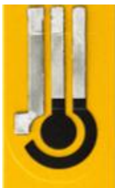
Figure 1. Model of chip electrochemical sensor LIG.
